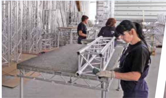
Truss frame systems undergoing final quality control inspection
