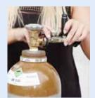
Ensure cylinder is standing securely, unscrew cylinder cap if applicable. Screw inflation valve on to cylinder valve by hand (do not use a tool!)
